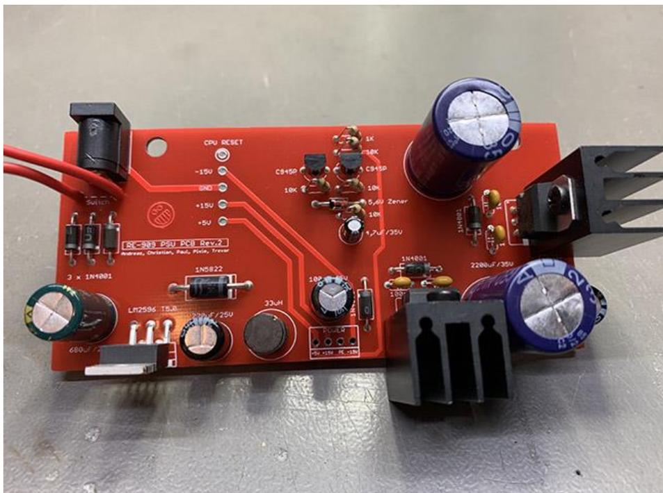
Use a piece of cable (approx. 12cm) and solder it to the bridge for the **on-off switch**. (Switch)
