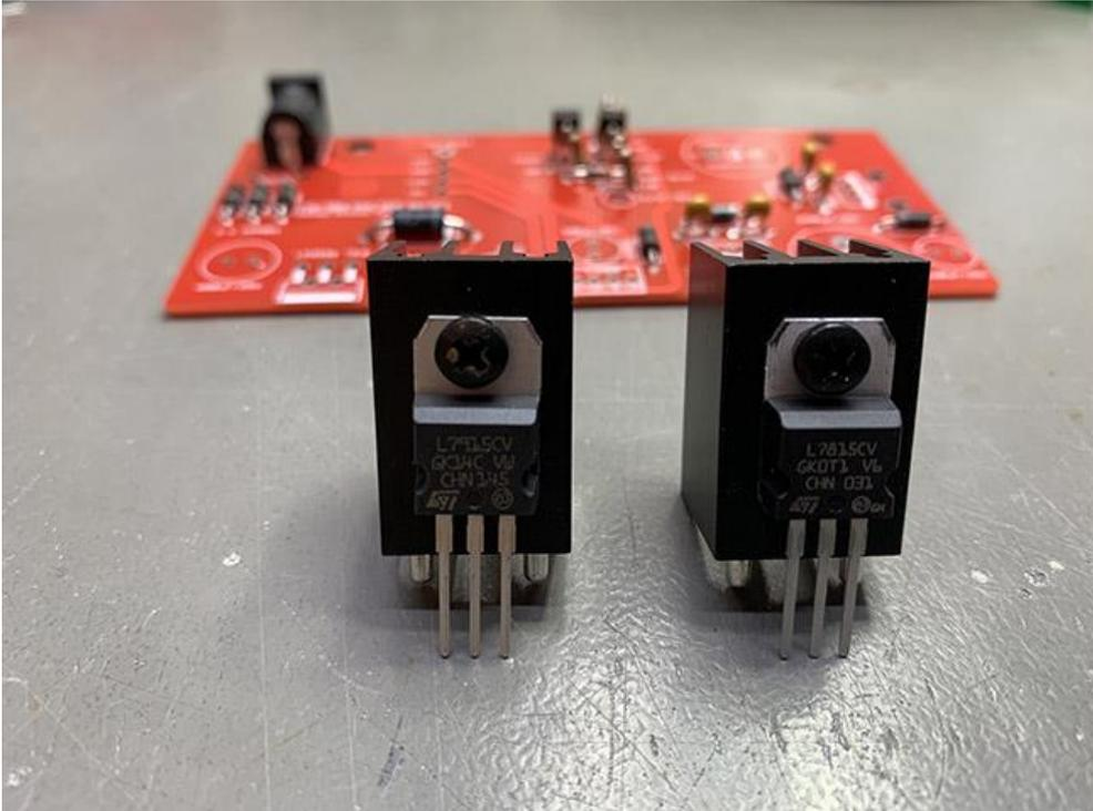
Now insert the voltage regulators with the heat sinks and solder them cleanly. **Always solder only ONE pin**, wait a short time and then solder the next pin. So you **avoid an overheating** of the voltage regulator! By the way, the LM2596 T5.0 regulator doesn't need a heat sink, but don't add too much heat when soldering! The pins of the two heat sinks **CAN** be soldered, but **not necessarily!**
