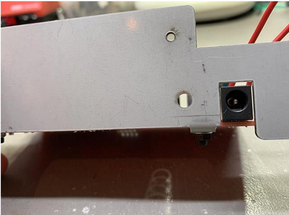
Position the board so that the power supply jack is centered in the opening of the bracket. Now your Safety PSU is ready for use in your RE-909!
