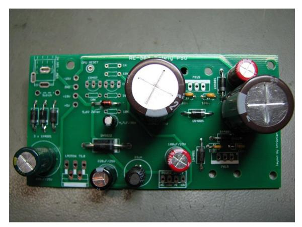
Now solder in the  $33\mu$ H inductance. There is no polarity here, the direction doesn't matter.
